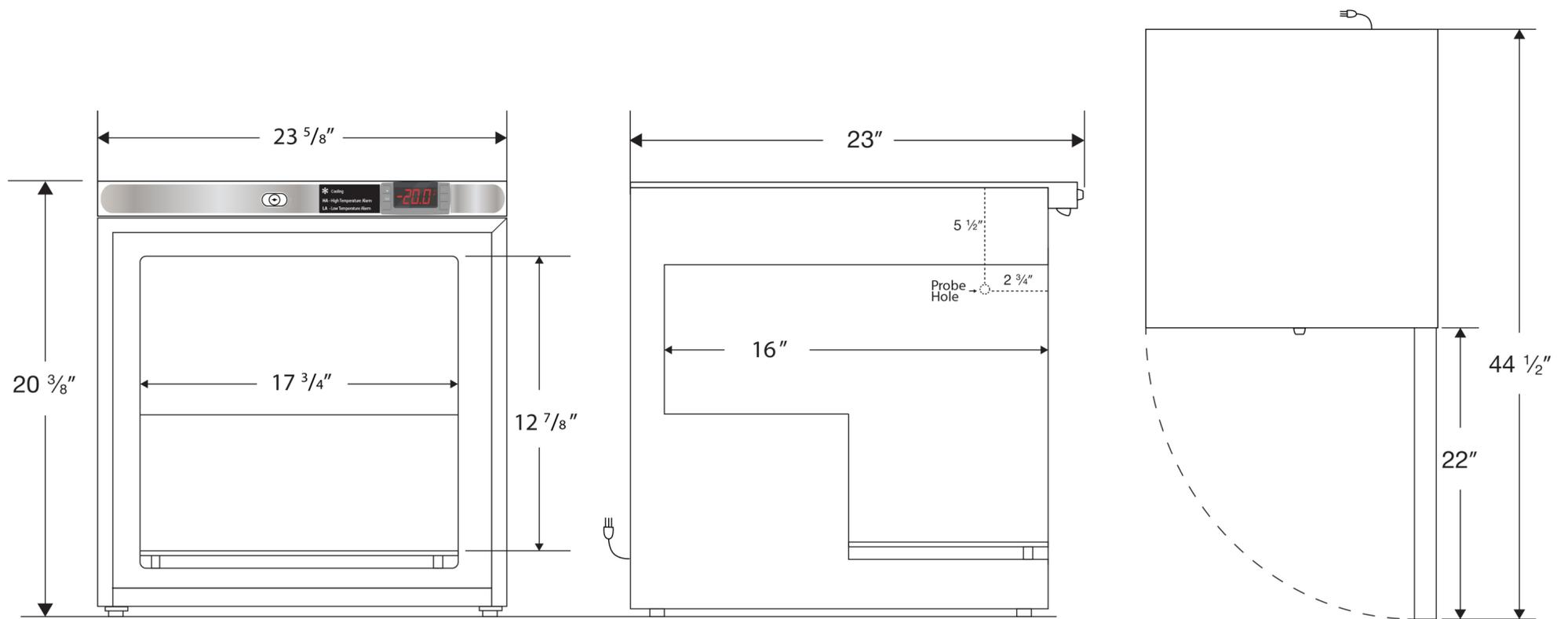
**Note:** This unit must have 4" clearance on sides and back for adequate ventilation
