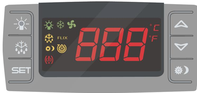
1. Press the **SET** button and the
